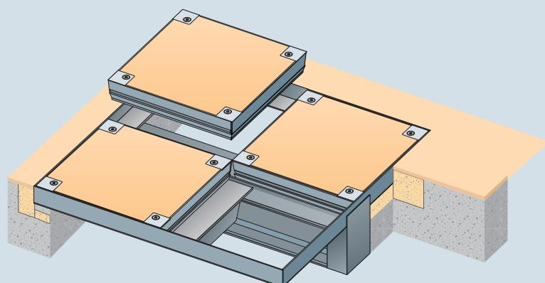
Cross section showing removable support beam and cross members (scale 1:5)
